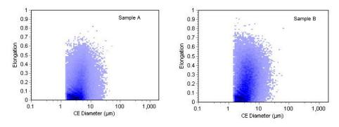
Figure 4: Scattergrams of CE Diameter vs. Elongation
