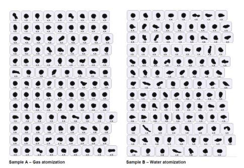
Figure 5: Example images of particles from around the modal size value (individual CE Diameter (µm)) indicated
