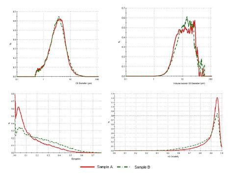
Figure 3: Overlays of some size and shape parameters. Samples A and B are very similar in terms of CE Diameter (both in number and volume weighting) but differ in terms of Elongation and HS Circularity
