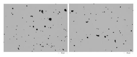
Figure 1: Field of view images of the two dispersed atomized metal samples with Sample A (left) and Sample B (right)
