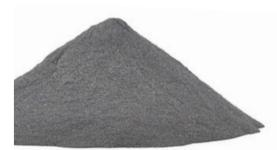
Powder metallurgy refers to the production and working of metals as fine powders which can be pressed and sintered to form objects.
