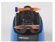
15 mL conical tubes x 2 (horizontally mounted)
