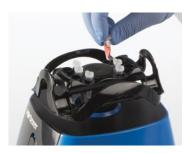
0.5 mL microfuge tubes x 6 (vertically mounted)
