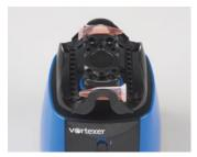
5 mL tubes x 2 (horizontally mounted in the same retention space as 15 mL)
