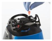
1.5/2 mL microfuge tubes x 4 (vertically mounted)
