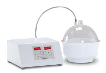
The ERWEKA VDT/S is a vacuum leak tester for blisters and other vacuum forms. With its compact size, the VDT is ideal for quality control during the packing and filling process. The ERWEKA VDT/S consists of two connected units - the main control unit with the integrated vacuum pump and the vacuum exsiccator (available in different sizes with 150, 200, 250 or 300 mm diameter).
