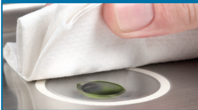
Ultra - Flat Prism and Sample Dish
