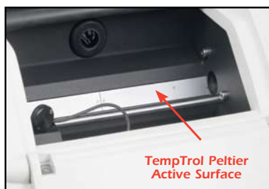
TempTrol heating and cooling Peltier transfer surface
