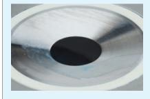
An improperly cleaned prism, where sample residue is left in the measurement well, can mix with a water zero or calibration fluid. This type of contamination during the calibration process will cause an error across all subsequent measurements.
