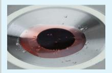
Many samples have air trapped inside them or are carbonated. These samples read well most of the time as long as air bubbles are not trapped between the prism surface and the sample. When this happens the operator gets an erroneous result often referred to as a flyer. These results are called flyers because the measured value is quite different from the expected measurment value.
