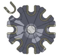
Inserts on the upper holders can be added or removed to accommodate the fit of different pipette widths
