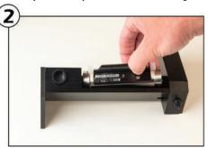
Place a 2.5mm or 5.0mm bore Polarimeter cell into the Rudolph FillStation™.
